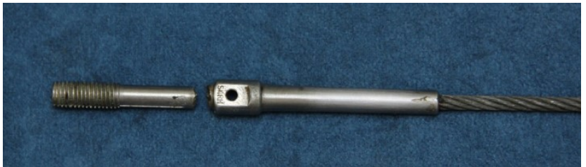
Failed terminal from Minicab GY-201 aircraft identified during inspection
